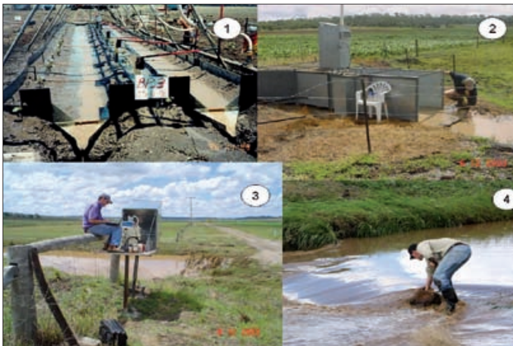
A range of approaches and scales were used to study movement of agricultural chemicals in cropping catchments; 1. rainfall simulator for detailed process studies, 2. monitoring runoff from paddock or contour bays, 3. sampling runoff from sub catchments and 4. collecting samples from creeks and rivers.
